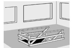
**Conclusion:** OSHA regulations state that "Employers shall provide and install all fall protection systems required before an employee begins work." Falling from heights is the leading cause of injury at job sites. Proper railing will add to a safe and compliant work place.
