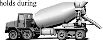
**Mechanical hazards** during equipment operations, such as handling of the load-out chute, can cause pinch point injuries to the hands and fingers, or being struck by swinging parts and falling material and equipment. Moving mixer parts also pose entanglement hazards to the operator.
